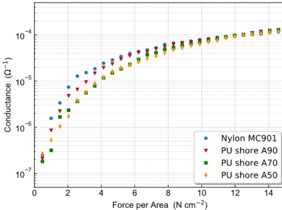
The response resulting from an actuation with the Nylon contact part (the hardest) is plotted as blue circles. For softer materials with a shore hardness between A90 and A50, a shift in the response is observed especially at lower actuation forces. This can be interpreted as a continuous deformation of the material under the applied force due to the different viscoelasticity of the polyurethanes.
