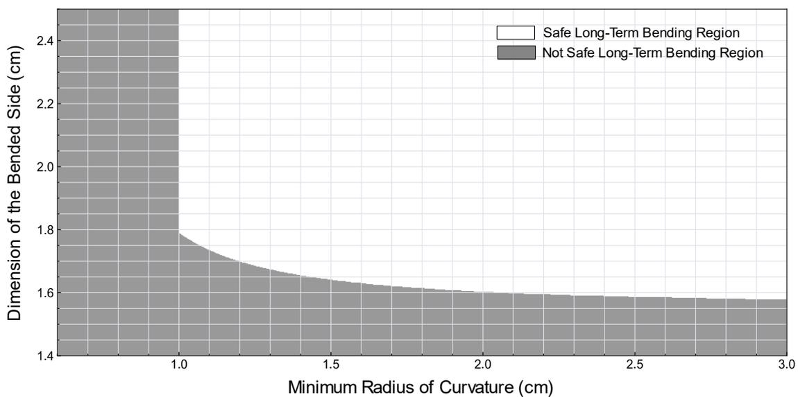
The white area of the graph represents the regime in which the TrueZero remains valid, which shows a minimum bending radius of around 1 cm. Please note that these are general and indicative values that have to be checked for a given application. As illustrated in the figure below, the sensor can be bent along its long side (L) as well as along its short side (W). The graph for the minimum bending radius is valid for both bending directions.
