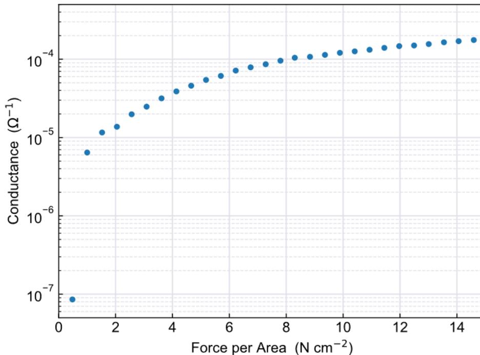
The reported force-conductance curve is measured from a model PFL-100010S with a cylindrical Nylon (MC901) actuator of 8 mm diameter, resulting in a total actuation area of 0.5 cm<sup>2</sup>. The readout signal as well as the main sensor parameters, such as the force range and the sensitivity, are influenced by many factors:
