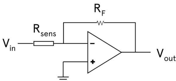
A transimpedance amplifier (TIA) converts the current flowing through the sensor ( $V_{in}/R_{sens}$ ) to a voltage signal ( $V_{out}$ ), providing a more ideal transfer function than a voltage divider.
