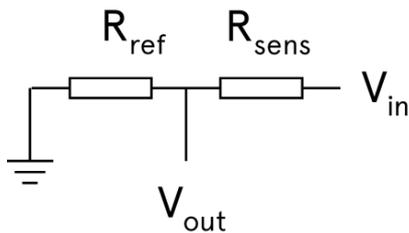
A voltage divider configuration is the simplest readout circuit to determine sensor resistance.
