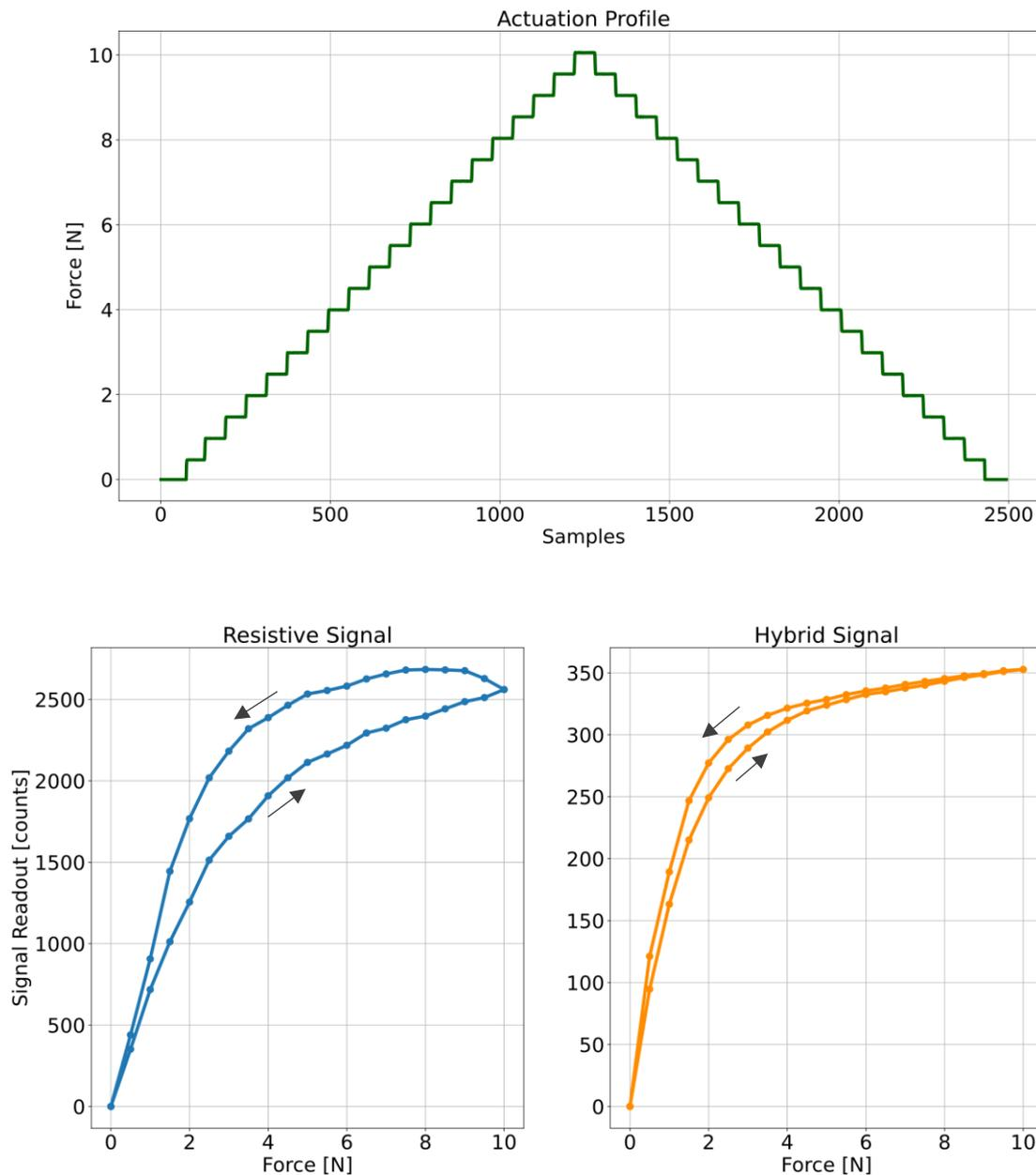
The sensor signal is determined for stepwise increasing/decreasing force levels ranging from 0 N to 10 N with 0.5 N force steps according to the depicted actuation profile.
