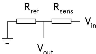
A voltage divider configuration is the simplest readout circuit to determine sensor resistance. Given that  $R_{ref}$  and  $V_{in}$  are known, the sensor resistance  $R_{sens}$  can be calculated by measuring the voltage drop  $V_{out}$  across the reference resistor  $R_{ref}$ .
