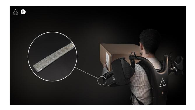
Munich, May 25, 2023 – The AGADEXO Shoulder is a semi-active exoskeleton for workers, which improves ergonomics by reducing stress on the shoulders during picking tasks. Suitable for use cases such as end-of-line logistics, manufacturing processes, and retailing, it has integrated tacterion's plyon® force sensors to detect grasping motions during picking activities.
